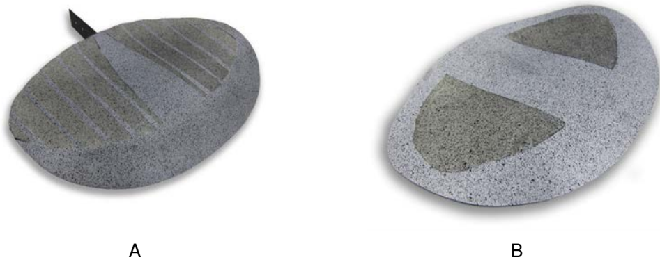
Figure 8-7. Isometric view of silicone membrane wings. A) Batten reinforced silicone membrane wing. B) Perimeter reinforced silicone membrane wing. Photos taken by Bradley LaCroix.
