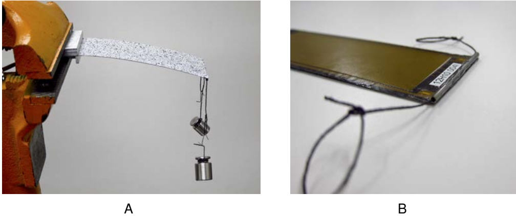
Figure 6-1. Cantilevered unimorph DIC setup. A) DIC setup with the unimorph cantilevered and the loads applied to the free end. B) M8528-P1 unimorph with the aluminum tube and string attached. Photos taken by Bradley LaCroix.
