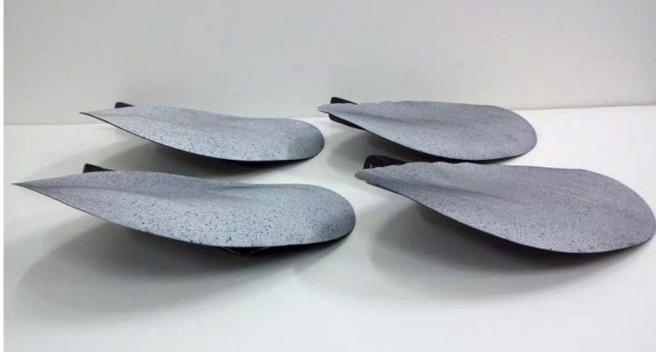
Figure 8-17. Rigid wing counterparts. The perimeter reinforced wings are shown on the left and the batten reinforced wings are shown on the right. Photo taken by Bradley LaCroix.
