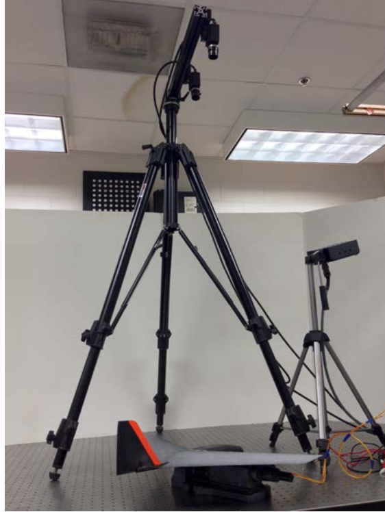
Figure 9-12. The workbench setup for MFC1. The DIC cameras are positioned above the aircraft and the aircraft is mounted to the table via a large vice. Photo taken by Bradley LaCroix.
