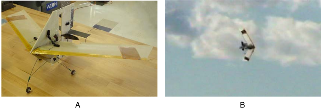
Figure 2-4. Micro air vehicle with MFC actuated roll control. Photos courtesy of Bilgen [39]. A) Completed MAV shown with MFCs. B) The same MAV during flight testing.
