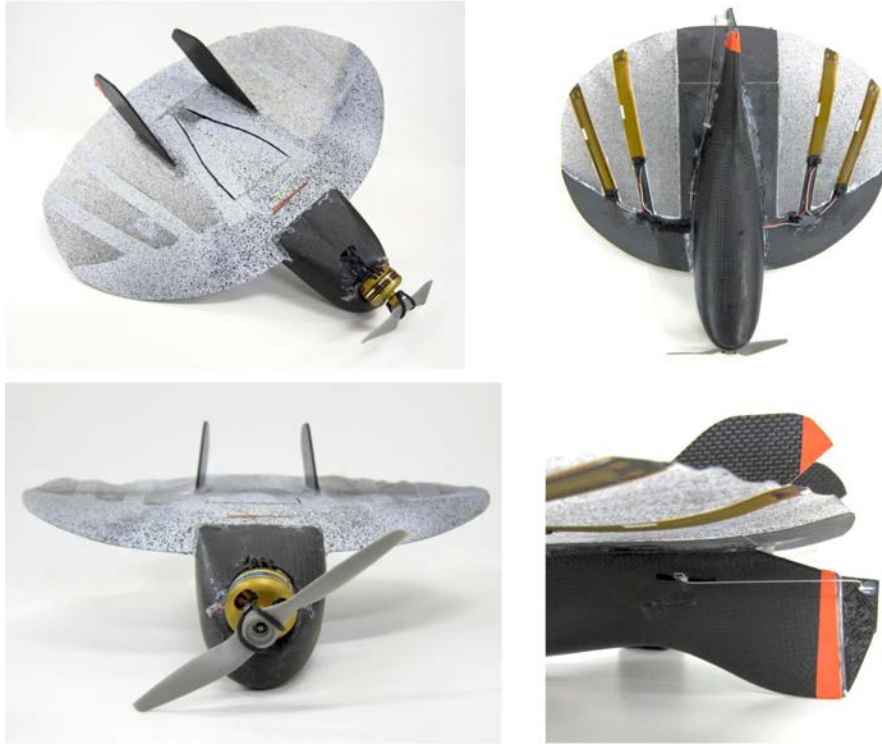
Figure 8-1. Images of the first MFC actuated MAV constructed under this research. Photos taken by Bradley LaCroix.
