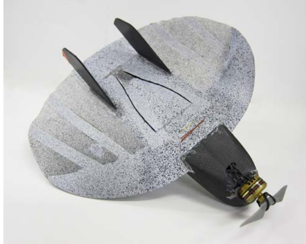
Figure 1-5. One of the first MAVs manufactured with MFCs. The membrane is ripstop polyester with a DIC speckle pattern applied. MFCs are applied to the underside of the battens. Photo taken by Bradley LaCroix.
