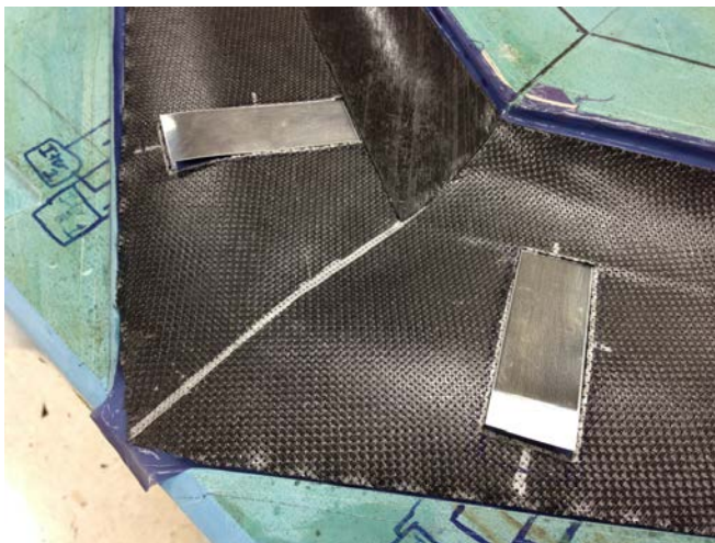
Figure 12-2. Manufacturing of the MFC13 wing. A) Steel substrate placed in the cutout section of MFC13 prior to curing. B) Picture of the MFC13 wing, post-cure. Photos taken by Bradley LaCroix.
