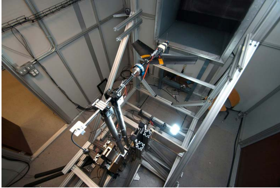
Figure 10-5. The overall wind tunnel setup. The DIC cameras are located below the aircraft. Photo taken by Bradley LaCroix.
