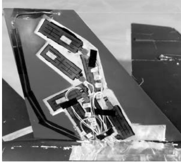
Figure 1-2. Application of piezoelectric materials on the tail of a model F/A-18 to reduce buffeting. Photo courtesy of NASA [16].
