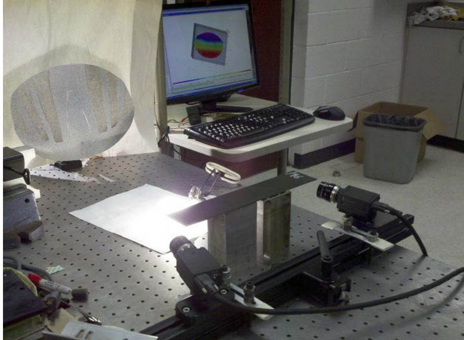
Figure 8-3. DIC setup for first MFC actuated MAV wing. Photo taken by Bradley LaCroix.
