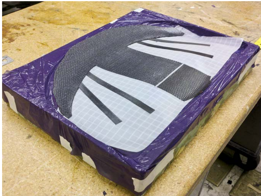
Figure 8-2. Manufacturing of the first MFC actuated MAV wing. Photo taken by Bradley LaCroix.
